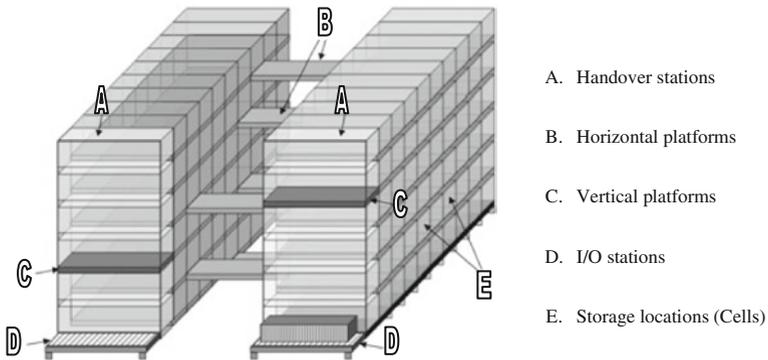
**Fig. 8.8** A schematic view of split-platform AS/RS (SP-AS/RS) (Modified after Hu et al. 2005)
