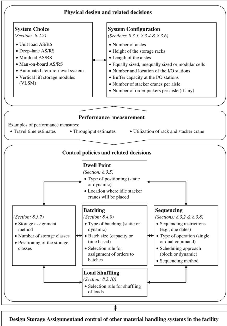
Fig. 8.5 Design of an AS/RS and related decisions (Modified after Roodbergen and Vis 2009)
