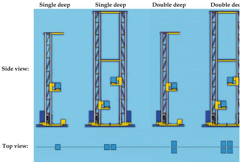
**Fig. 8.4** Some common types of stacker cranes in AS/RSs (Courtesy of Stöcklin Logistik AG)
