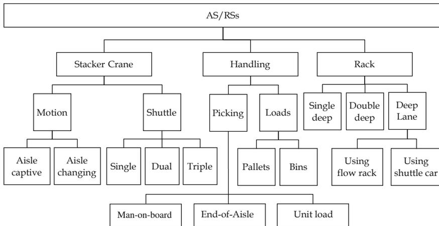
**Fig. 8.3** Various system concepts for AS/RSs (Modified after Roodbergen and Vis 2009)
