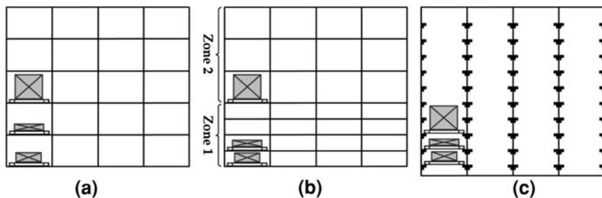
**Fig. 8.9** Structure of the rack with **a** Equal sized, **b** Unequal sized and **c** Modular cells
