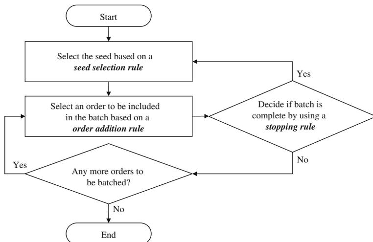
**Fig. 8.12** Common procedure for order-batching Heuristics (Modified after Pan and Liu 1995; Roodbergen and Vis 2009)
