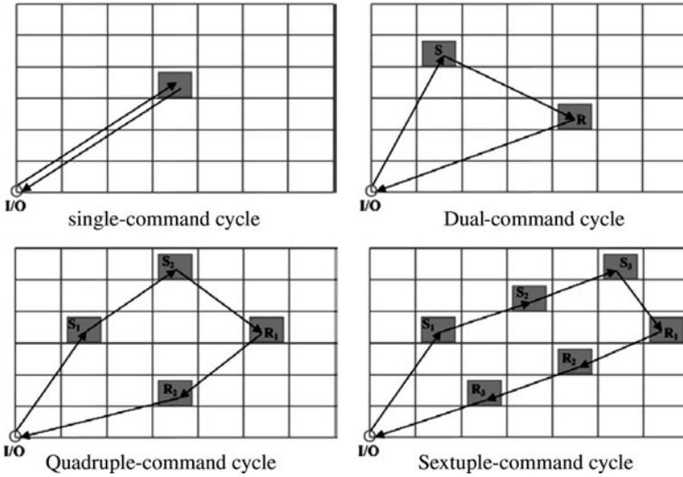
Fig. 8.7 Different command cycles of the stacker crane
