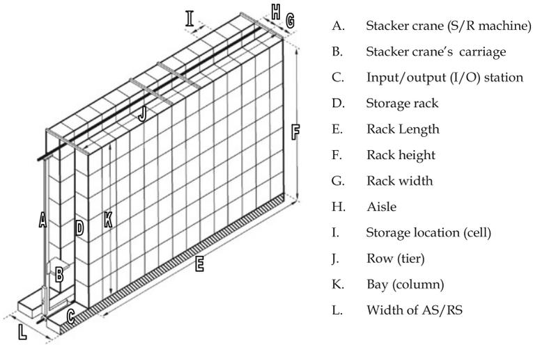
Fig. 8.14 Generic Structure and principal constituents of an AS/RS
