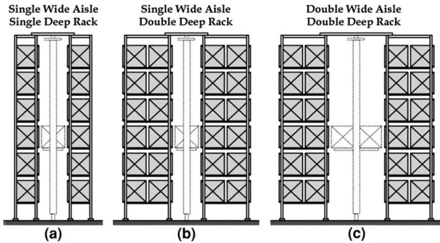
Fig. 8.15 Some common types of rack structures in AS/RSs. **a** Single wide aisle, single deep rack. **b** Single wide aisle, double deep rack. **c** Double wide aisle, double deep rack
