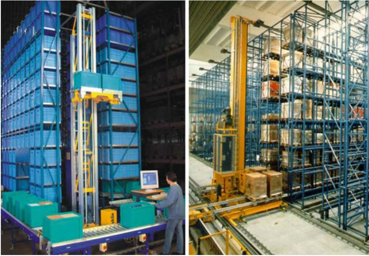
**Fig. 8.2** Automated storage and retrieval systems (Courtesy of Stöcklin Logistik AG)
