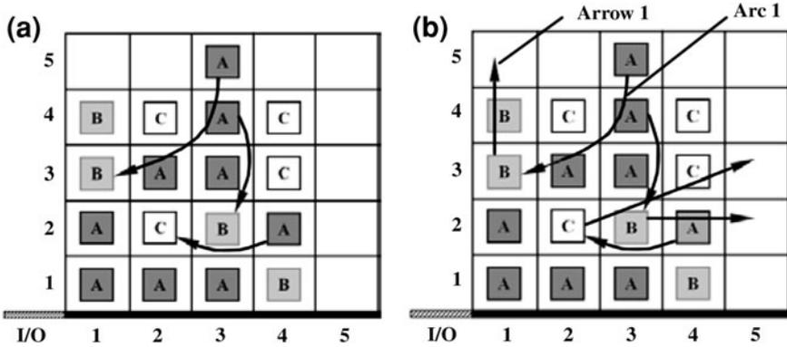
Fig. 8.13 (a, b) Matching for load shuffling in an AS/RS (Modified after Muralidharan et al. 1995)
